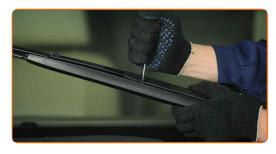
Remove the blade from the wiper arm.
