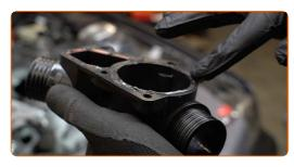
23 Install the new thermostat housing.
