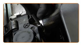
Remove the coolant reservoir cap.
