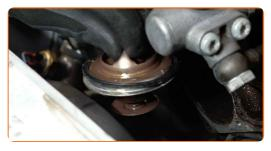
Clean the thermostat housing mounting seat. Use a flat screwdriver. Use a seal scraper. Use all-purpose cleaning spray.
