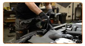
5 Unscrew the coolant reservoir cap.
