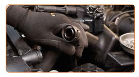
Unscrew the fastener of the chassis (ground) terminal of the ignition coils. Use a drive socket #8. Use a ratchet wrench.
