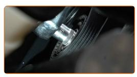
Pull aside the AC compressor belt tensioner pulley. Use a drive socket #13.
