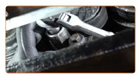
Remove the AC compressor belt.
