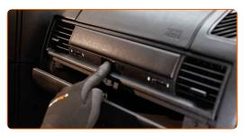
Unscrew the glove box fastening screws. Use a Phillips screwdriver. Use a flat screwdriver.
