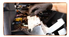
Remove the fasteners of the air duct housing. Use a clip removal tool.
