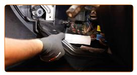
17 Install the air duct housing fasteners.
