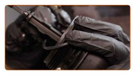
Install the new oil filter to the mounting seat on the filter cover.
