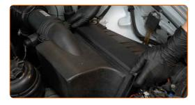
Remove the air filter housing.
