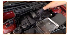
Screw the cap. Use the 86/16 F socket. Use a torque wrench. Tighten it to 25 Nm torque.
