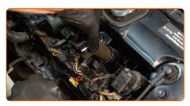
Plug in the ignition coil connector.
