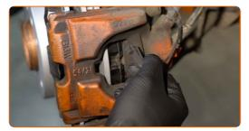
Disconnect the brake pads wear sensor.
