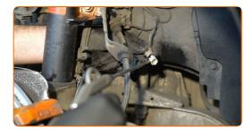
Connect the brake pad wear sensor plug.
