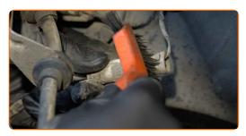
Disconnect the brake pad wear sensor plug.
