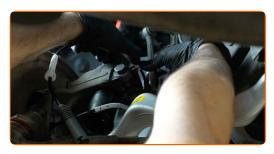
17 Attach the ABS sensor connector.
