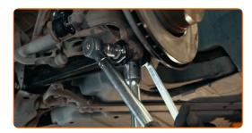
Tighten the fastener connecting the control arm to the subframe. Use a drive socket #18. Use a torque wrench. Tighten it to 77 Nm torque.
