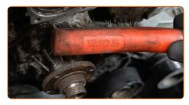
Unscrew the water pump fasteners. Use a drive socket #10. Use a ratchet wrench.
