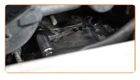
18 Remove the thermostat housing.
