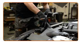
5 Unscrew the coolant reservoir cap.
