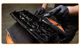
Treat the engine valve cover mounting seat. Use a sealant.
