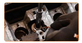
Raise a little the wiring of the ignition coils and move it aside. Use a flat screwdriver.
