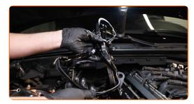
Clean the engine valve cover mounting seat. Use a seal scraper. Use all-purpose cleaning spray.
