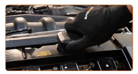
Unplug the connectors from the ignition coils. Use a crowbar.
