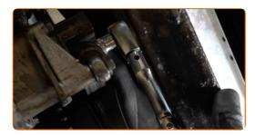
12 Install the AC compressor belt.
