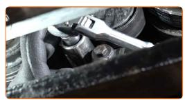
Remove the AC compressor belt.
