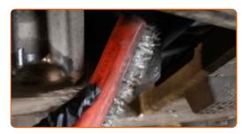
Unscrew the drain plug. Use a drive socket #19. Use a ratchet wrench. 11
