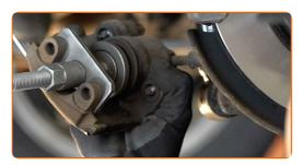
Treat the back side of the new brake pads. Use anti-squeal paste.
