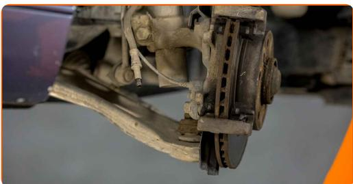
Replacement: brake caliper – BMW 3 Convertible (E36). Tip from AUTODOC:
