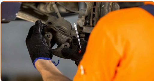
**16** Unscrew the brake hose from the brake caliper. Use a flare nut spanner #14.
