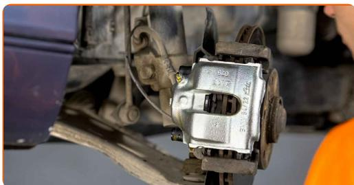
**24** Bleed the brake caliper system. Without starting the engine, press the brake pedal several times until you feel significant resistance.
