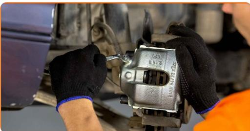
**23** Connect the brake bleeder kit to the brake bleeder screw.
