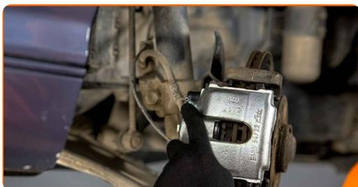
Replacement: brake caliper – BMW 3 Convertible (E36). Tip:
