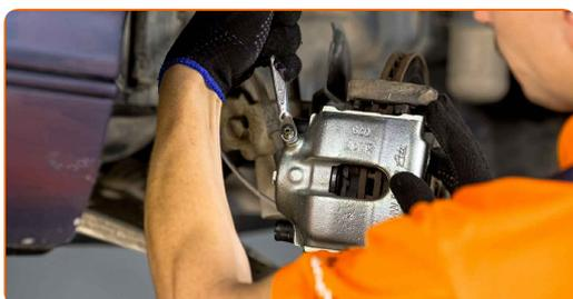
**27** Clean dirt from the brake hose bolt. Use a brake cleaner.
