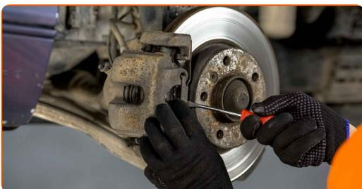
**8** Remove the dust boot caps of the brake caliper guide pins. Use a crowbar.
