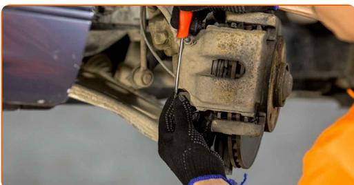
**9** Clean the area where the brake hose is connected to the caliper, and the guide pins area. Use a wire brush. Use a brake cleaner.
