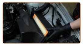
o Press the air filter cover clips into place.
