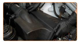
Remove the air filter housing.
