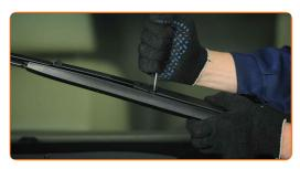
A Remove the blade from the wiper arm.
