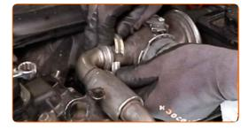
Tighten the clamp of the EGR cooler pipe. Use a drive socket #7. Use a ratchet wrench.
