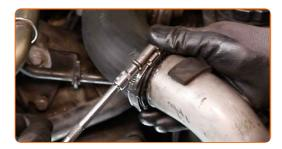
Clean the mounting seats of the coolant hose. Use all-purpose cleaning spray.
