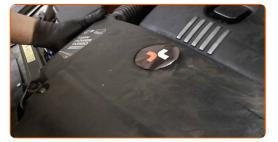
Screw in the fasteners of the air distribution housing assembly. Use a drive socket #12. Use a ratchet wrench.
