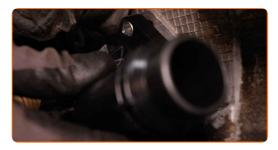
Tighten the thermostat housing fasteners. Use a drive socket #10. Use a torque wrench. Tighten it to 9 Nm torque.
