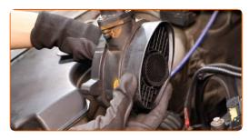
Install a new mass air flow sensor.
