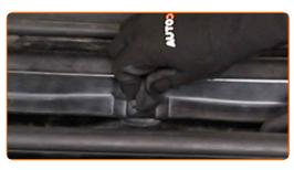
Install the engine cover and secure it.
