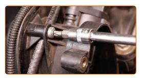
Remove the mass air flow sensor.
