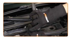
Install the cabin filter to its mounting seat.
