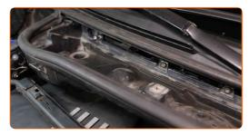
Screw in the fasteners of the cabin filter housing. Use Torx T30. Use a ratchet wrench.
