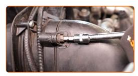
17 Remove the air duct.
