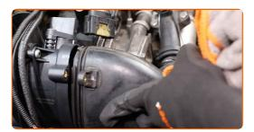
Tighten the fasteners that connect the air duct to the MAF sensor. Use HEX No.H5. Use a torque wrench. Tighten it to 5 Nm torque.
