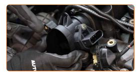
Tighten the MAF sensor fasteners. Use Torx T25. Use a torque wrench. Tighten it to 8 Nm torque.
