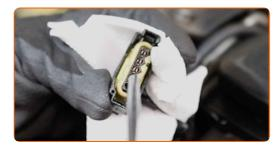
28 Attach the mass air flow sensor connector.
