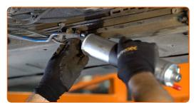
Tighten the fastening clamps of the fuel filter pipes. Use a drive socket #7. Use a ratchet wrench.
