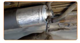
Install the fuel filter fastening bracket.
