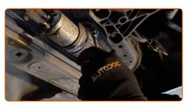
9 Remove the fuel filter fastening bracket.
