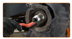
Install the new wheel hub with a bearing. Use a drive socket #46. Use a hammer.
