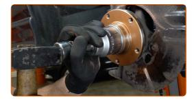
26 Install the brake disc.
