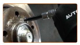
Remove the brake disc.
