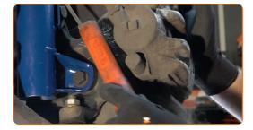
Unscrew the caliper bracket fastening. Use a drive socket #16. Use a tap wrench.
