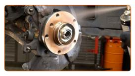
Install the cap of the hub nut. Use a drive socket #46. Use a hammer.
