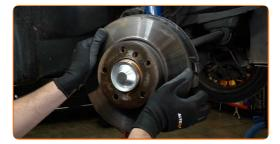
Tighten the brake disc fastening. Use HEX No.H6. Use a torque wrench. Tighten it to 9 Nm torque.
