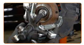
Pull the bearing inner race out of the wheel hub. Use a universal puller.
