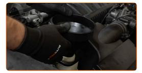
Pour coolant in the coolant reservoir.
