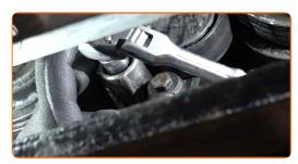
Remove the AC compressor belt.
