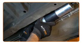
Screw in the fuel filter mounting bracket. Use HEX No.H5. Use a ratchet wrench.
