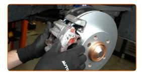
Install the brake caliper retaining spring.
