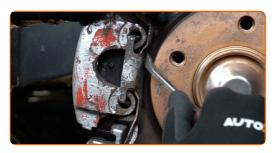
Remove the brake caliper.
