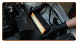
9 Press the air filter cover clips into place.
