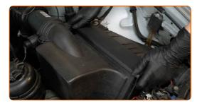
Remove the air filter housing.
