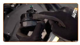
Screw the new filter into its place.
