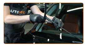
Remove the blade from the wiper arm.
