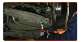
20 21 Treat the shock absorber fasteners. Use copper grease.
