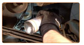
Pull down the suspension control arm. Use a crowbar.
