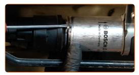
Loosen the fastening clamp of the fuel filter pipe. Use a flat screwdriver.
