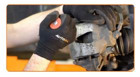
10 Remove the brake caliper.
