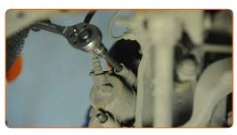
Remove the brake caliper.
