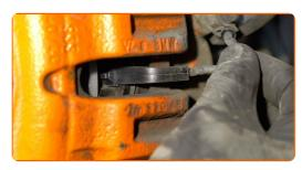
Treat the surface where the brake disc contacts the wheel rim. Use copper grease.
