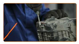
Reinstall the air filter housing.
