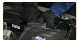
Screw in the clamp that connects the air filter hose to the throttle body. Use a flat screwdriver.
