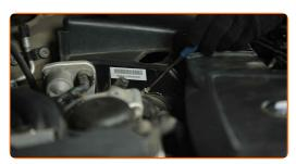
Screw the filter housing fastening bolts. Use a drive socket #10. Use a ratchet wrench.
