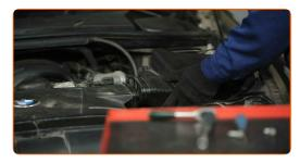
Unscrew the filter housing fastening bolts. Use a drive socket #10. Use a ratchet wrench.
