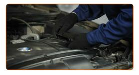
Unplug the mass air flow sensor connector. Use a flat screwdriver.
