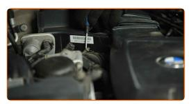
Disconnect the air intake pipe from the air filter housing. Use a flat screwdriver.
