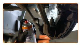
Treat the ABS sensor fastener. Use a multipurpose grease. Use a flat screwdriver.
