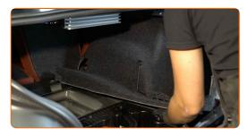
Screw in the fastener of the boot side lining. Use Torx T40. Use a ratchet wrench.
