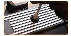
Install the engine cover and secure it.
