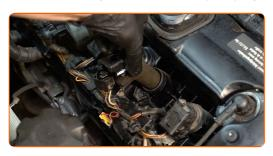
Plug in the ignition coil connector.
