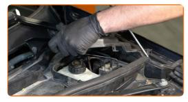
Detach the connectors from the climate control sensors.
