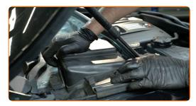
Attach the cable duct to the upper part of the microfilter housing.
