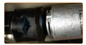
Install the snap ring of the fuel pressure regulator's retainer clip.
