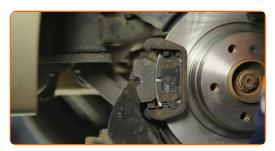
Remove the brake pads retaining clips. Use a flat screwdriver.
