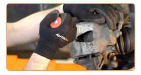
10 Remove the brake caliper.
