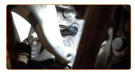
Tighten the fastener that connects the ABS sensor to the steering knuckle. Use HEX No.H5. Use a torque wrench. Tighten it to 13 Nm torque.
