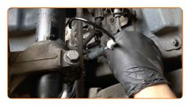
Connect the ABS sensor wiring.
