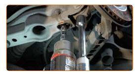
Remove the support from under the stub axle.
