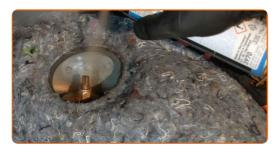
Install the mount cap on the shock absorber upper fastener.
