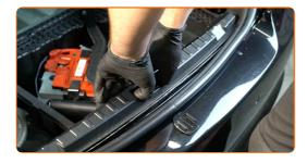
Unscrew the fastener of the boot side lining. Use a clip removal tool. Use Torx T40. Use a ratchet wrench.
