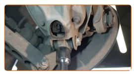
Screw in the lower fastener of the shock absorber. Use a drive socket #14. Use a ratchet wrench.
