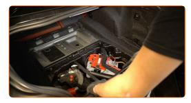
Screw in the fastener of the central protective plastic panel. Use a Phillips screwdriver. Use Torx T40. Use a ratchet wrench.
