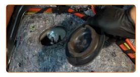
Loosen the upper fastener of the shock absorber. Use a shock absorber socket DDNº6. Use a drive socket #16. Use a ratchet wrench.
