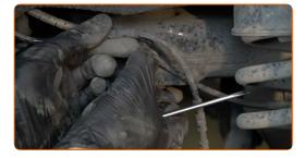
Unscrew the wheel arch cover fasteners. Use a drive socket #10. Use a ratchet wrench.
