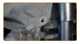
Disconnect the brake pad wear sensor plug.
