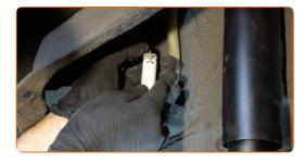
Install the wheel arch cover to its mounting seat. Screw in the fasteners. Use a drive socket #10. Use a ratchet wrench.
