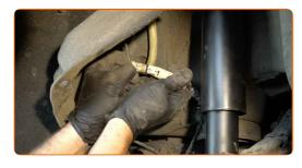
Connect the brake pad wear sensor plug.
