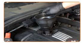
Pour oil into the engine through the filler. Required amount of oil: 6.5 L.
