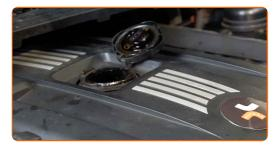
Tighten the oil filler cap.
