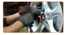
Lower the car and working in a cross order, tighten the wheel bolts. Use wheel impact socket #17. Use a torque wrench. Tighten it to 120 Nm torque.
