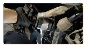
Screw the fasteners of the ball joint. Use a drive socket #21. Use a ratchet wrench.
