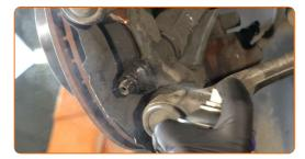
Unscrew the ball joint fastening to the steering knuckle. Use a combination spanner #21. Use HEX No.H6. Use a ratchet wrench.
