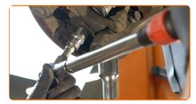
18 Remove the support from under the arm.
