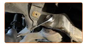
9 Remove the front fastener of the control arm.
